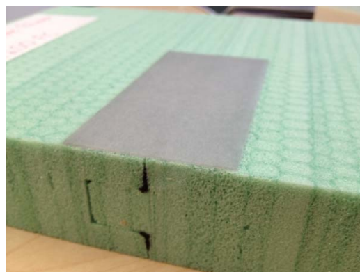
Figure 04.06 - Tongue and groove connection with adhesive type - Samples 3,4.
