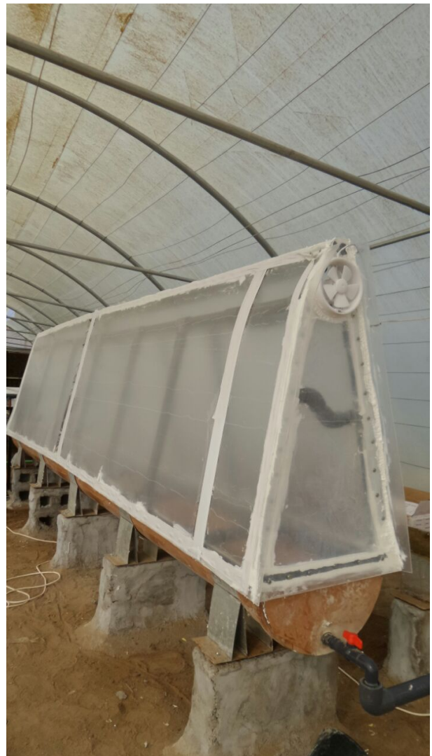
Figure 05.76: Acrylic sheets used for constructing the tent.
