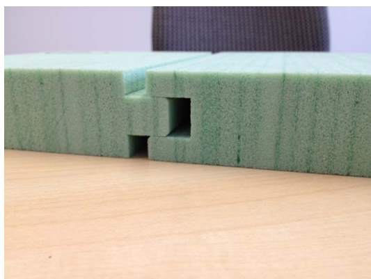
Figure 04.04 - Open and closed tongue and groove connection - Sample 7.
