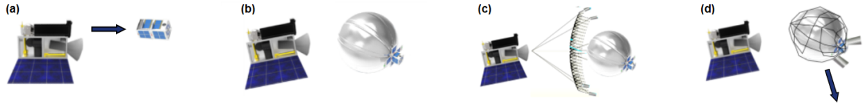
Fig. 1: Net Experiment. This figure shows the sequence in the net experiment: (a) DS-1 CubeSat ejection, (b) balloon inflation, (c) net capture, (d) deorbiting.
